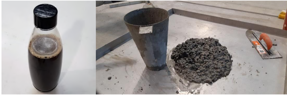
Figure 6 - Footage from the effects of newly proposed chemical admixture on the fresh state properties of concrete made by recycled aggregate.
