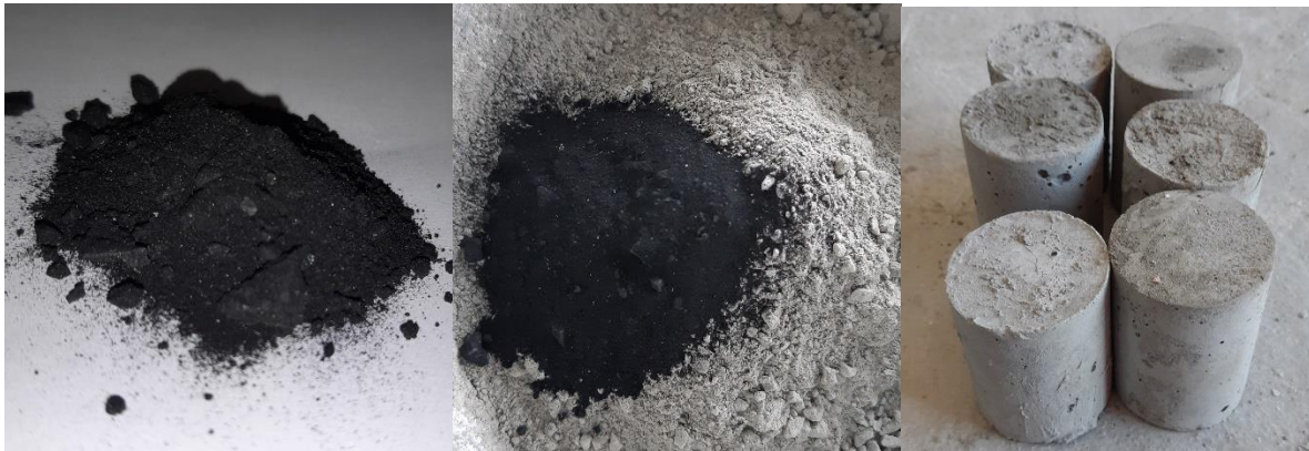
Figure 10 From left to right: filter dried graphene oxide - mix portion - cured samples
