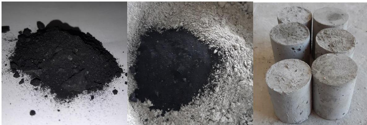
Figure 2 From left to right: filter dried graphene oxide - mix portion - cured samples
