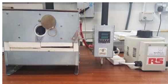
Figure 3 – Kiln with transformer
